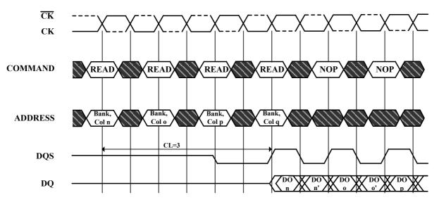
DO n, etc. =Data Out from column n, etc. n', etc. =the next Data Out following DO n, etc. according to the programmed burst order Burst Length=2,4 or 8 in cases shown. If burst of 4 or 8, the burst is interrupted Reads are to active rows in any banks
