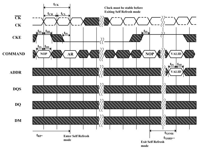
\* = Device must be in the "All banks idle" state prior to entering Self Refresh mode \*\* = tXSNR is required before any non-READ command can be applied, and tXSRD (200 cycles of CK) is required before a READ command can be applied.
