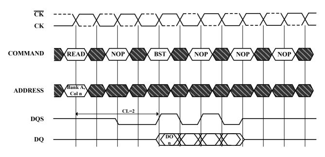
Figure 12. Terminating a Read Burst Required CAS Latencies (CL=2)
