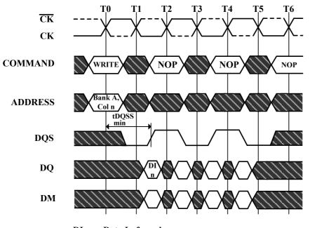
DI n = Data In for column n 3 subsequent elements of Data In are applied in the programmed order following DI n A non-interrupted burst of 4 is shown A10 is LOW with the WRITE command (AUTO PRECHARGE disabled)
