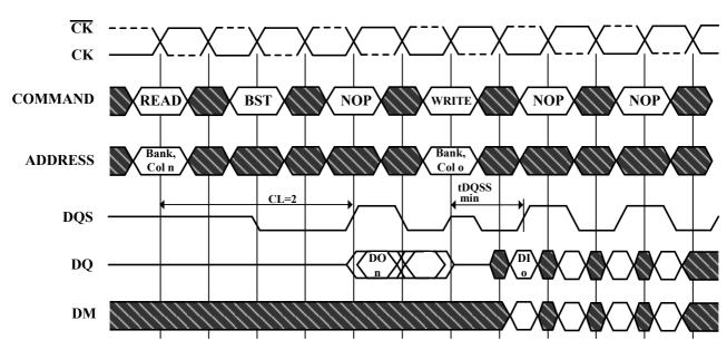
Figure 13. Read to Write Required CAS Latencies (CL=2)
