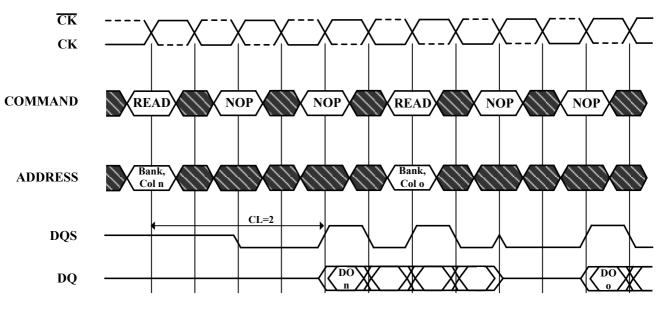
DO n (or o)=Data Out from column n (or column o) Burst Length=4
