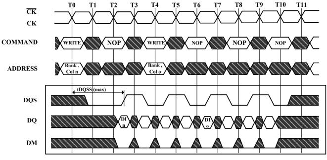
DI n , etc. = Data In for column n,etc. 3 subsequent elements of Data In are applied in the programmed order following DI n 3 subsequent elements of Data In are applied in the programmed order following DI o Non-interrupted bursts of 4 are shown DM= UDM & LDM
