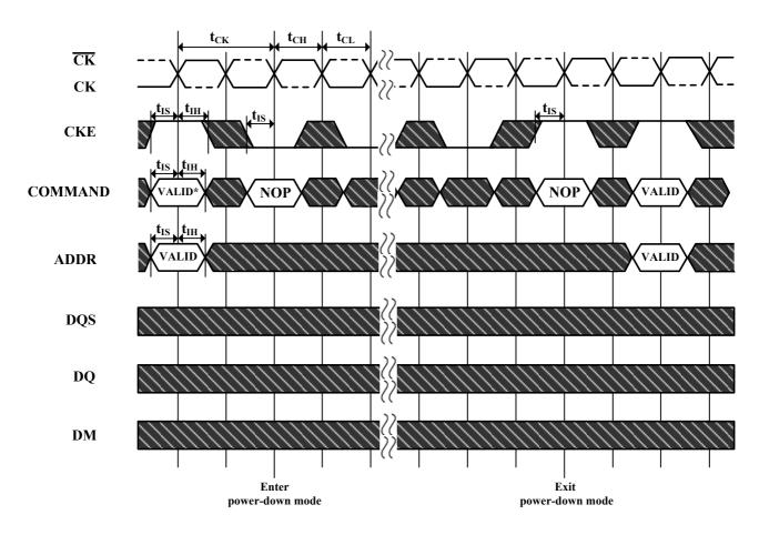
No column accesses are allowed to be in progress at the time Power-Down is entered \*=If this command is a PRECHARGE ALL (or if the device is already in the idle state) then the Power-Down mode shown is Precharge Power Down. If this command is an ACTIVE (or if at least one row is already active) then the Power-Down mode shown is active Power Down.
