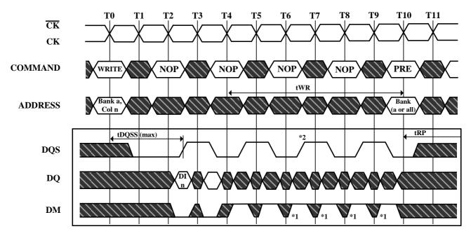
An interrupted burst of 4 or 8 is shown, 2 data elements are written tWR is referenced from the first positive CK edge after the last Data In Pair
