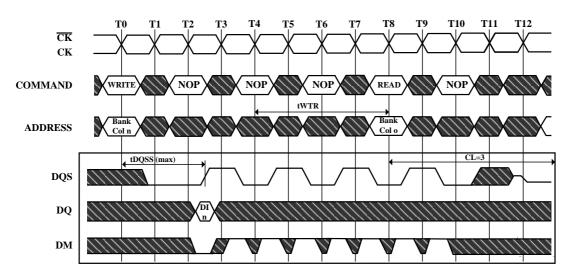
An interrupted burst of 8 is shown, 1 data elements are written
