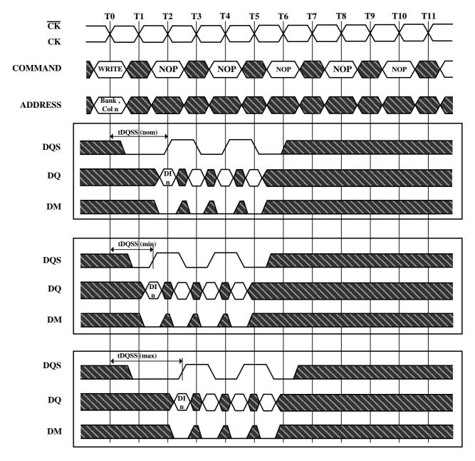
3 subsequent elements of Data are applied in the programmed order following DI n
