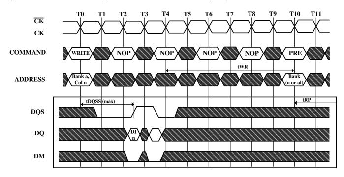
${f 1}$  subsequent elements of Data In are applied in the programmed order following DI n A non-interrupted burst of  ${f 2}$  is shown
