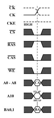
CA=Column Address BA=Bank Address EN AP=Enable Autoprecharge DIS AP=Disable Autoprecharge
