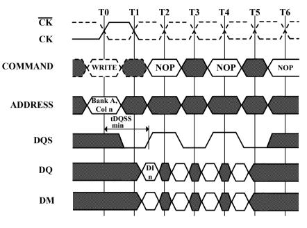
DI n = Data In for column n 3 subsequent elements of Data In are applied in the programmed order following DI n
