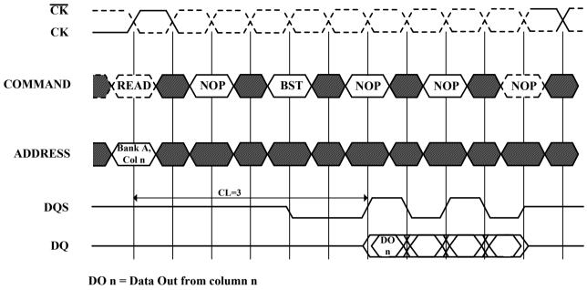
Cases shown are bursts of 8 terminated after 4 data elements 3 subsequent elements of Data Out appear in the programmed order following DO n
