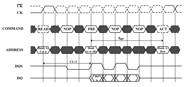
Figure 15. Read to Precharge Required CAS Latencies (CL=2)
