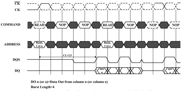
3 subsequent elements of Data Out appear in the programmed order following DO n (and following DO o)
