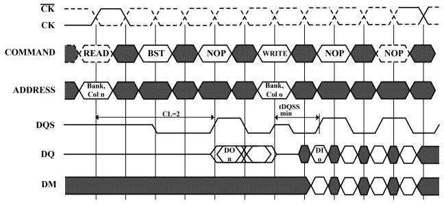
Figure 14. Read to Write Required CAS Latencies (CL=2)
