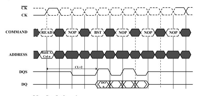
Figure 13. Terminating a Read Burst Required CAS Latencies (CL=2)
