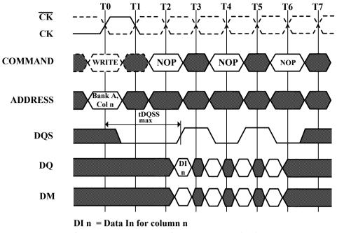
**3** subsequent elements of Data In are applied in the programmed order following DI n
