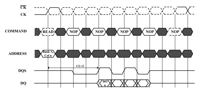
DO n=Data Out from column n Burst Length=4 3 subsequent elements of Data Out appear in the programmed order following DO n
