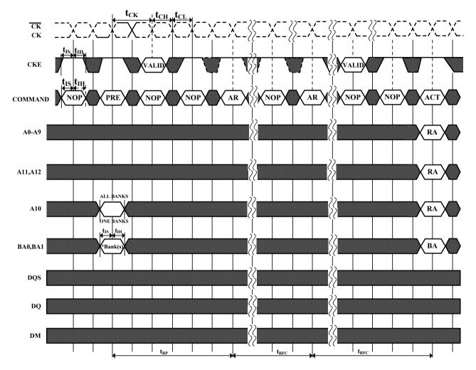
\*= "Don't Care", if A10 is HIGH at this point; A10 must be HIGH if more than one bank is active (i.e., must precharge all active banks) PRE = PRECHARGE, ACT = ACTIVE, RA = Row Address, BA = Bank Address, AR = AUTOREFRESH NOP commands are shown for ease of illustration; other valid commands may be possible after tRFC DM, DQ and DQS signals are all "Don't Care" /High-Z for operations shown
