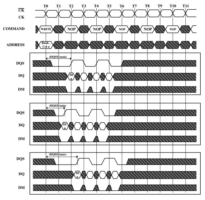
3 subsequent elements of Data are applied in the programmed order following DI n
