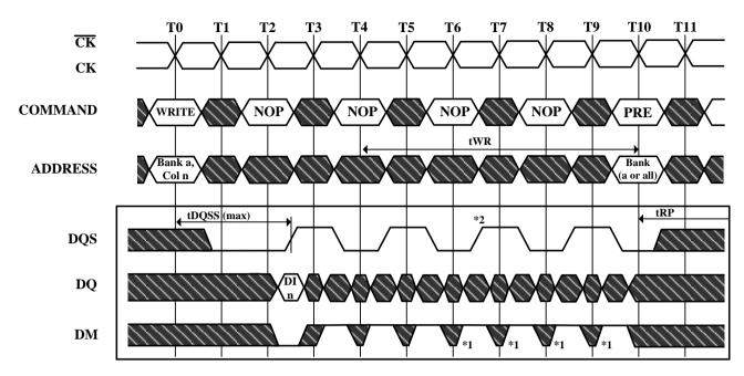
An interrupted burst of 4 or 8 is shown, 1 data element is written
