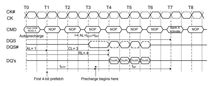
Figure 39. Burst read operation with auto precharge followed by activation to the same bank (t<sub>RC</sub> Limit): RL=5(AL=2, CL=3, internal t<sub>RCD</sub>=3, BL=4, t<sub>RTP</sub>≦2 clocks)
