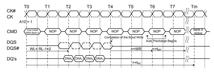
Figure 41. Burst write with auto-precharge (t<sub>RC</sub> Limit): WL=2, WR=2, BL=4, t<sub>RP</sub>=3
