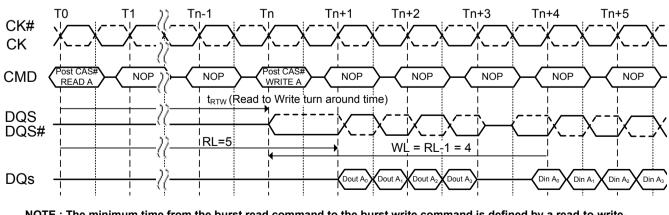
NOTE : The minimum time from the burst read command to the burst write command is defined by a read-to-writeturn-around-time, which is 4 clocks in case of BL = 4 operation, 6 clocks in case of BL = 8 operation.
