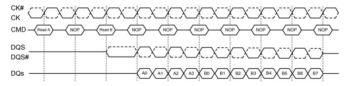
NOTE 1: Read burst interrupt function is only allowed on burst of 8. Burst interrupt of 4 is prohibited. NOTE 2: Read burst of 8 can only be interrupted by another Read command. Read burst interruption by Write
