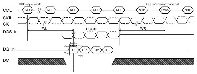
NOTE 1: For proper operation of adjust mode, WL = RL - 1 = AL + CL - 1t<sub>CK</sub> and t<sub>DS</sub>/t<sub>DH</sub> should be met as shown in the figure.
