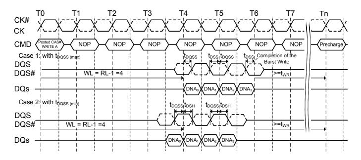
Figure 25.2. Burst write operation: RL=3 (AL=0, CL=3), WL=2, BL=4
