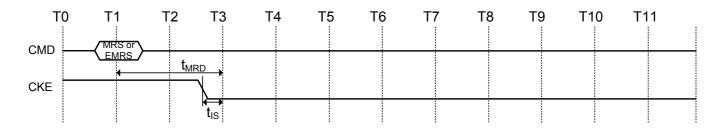
Figure 46. Asynchronous CKE LOW event
