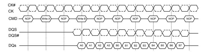
NOTE 1: Write burst interrupt function is only allowed on burst of 8. Burst interrupt of 4 is prohibited.
