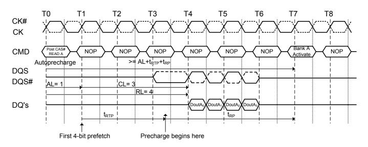
Figure 32.3. Burst read operation with auto precharge followed by activation to the same bank ( $t_{RC}$  Limit): RL=5(AL=2, CL=3, internal  $t_{RCD}$ =3, BL=4,  $t_{RTP}$  2 clocks)
