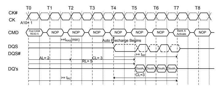
Figure 33.1. Burst write with auto-precharge (t<sub>RC</sub> Limit): WL=2, WR=2, BL=4, t<sub>RP</sub>=3
