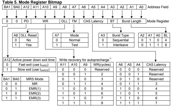
Note 1:.For DDR2-800, WR (write recovery for autoprecharge) min is determined by  $t_{CK}$  (avg) max and WR max is determined by  $t_{CK}$ (avg) min. WR [cycles] = RU { $t_{WR}$ [ns]/ $t_{CK}$ (avg)[ns]}, where RU stands for round up. The mode register must be programmed to this value. This is also used with  $t_{RP}$  to determine  $t_{DAL}$ .
