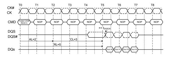
Figure 20.2. Burst read operation: RL=3 (AL=0, CL=3, BL=8)
