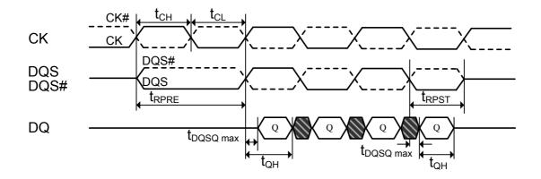
Figure 20.1. Burst read operation: RL=5 (AL=2, CL=3, BL=4)
