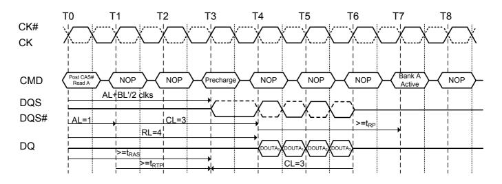
Figure 30.2.Burst read operation followed by precharge: (RL=4, AL=1, CL=3, BL=8, t<sub>RTP</sub> 2 clocks)
