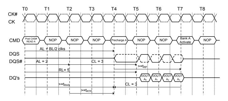
Figure 30.4. Burst read operation followed by precharge: (RL=6, AL=2, CL=4, BL=4, t<sub>RTP</sub> 2 clocks)
