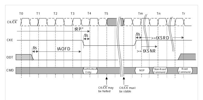
\* = Device must be in the "All banks idle" state to entering Self Refresh mode.
