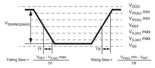
AC input test signal waveform
