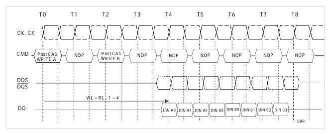
The seamless burst write operation is supported by enabling a write command every BL / 2 number of clocks. This operation is allowed regardless of same or different banks as long as the banks are activated.
