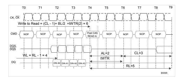
The minimum number of clocks from the burst write command to the burst read command is (CL - 1) + BL/2 + tWTR
