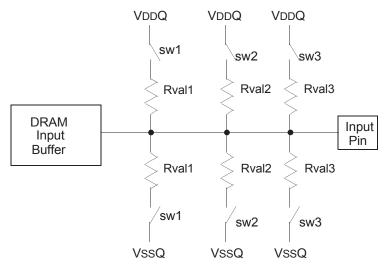
Switch (sw1, sw2, sw3) is enabled by ODT pin.
