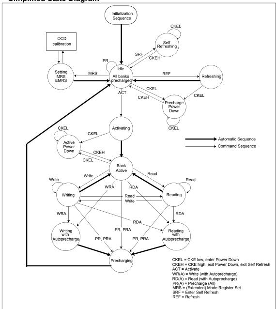
Note: Use caution with this diagram. It is intended to provide a floorplan of the possible state transitions and the commands to control them, not all details. In particular situations involving more than one bank, enabling/disabling on-die termination, Power Down entry/exit - among other things - are not captured in full detail.
