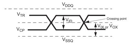
NOTE 1  $V_{ID(AC)}$  specifies the input differential voltage  $|V_{TR} - V_{CP}|$  required for switching, where  $V_{TR}$  is the true input signal (such as CK, DQS, LDQS or UDQS) and  $V_{CP}$  is the complementary input signal (such as  $\overline{CK}$ ,  $\overline{DQS}$ ,  $\overline{LDQS}$  or  $\overline{UDQS}$ ). The minimum value is equal to  $V_{IH(AC)} - V_{IL(AC)}$ .
