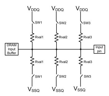
Switch (sw1, sw2, sw3) is enabled by ODT pin. Selection among sw1, sw2, and sw3 is determined by "Rtt (nominal)" in EMR. Termination included on all DQs, DM, DQS, DQS#, RDQS and RDQS# pins
