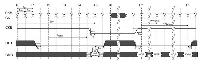
NOTE 1 Device must be in the "All banks idle" state prior to entering Self Refresh mode.
