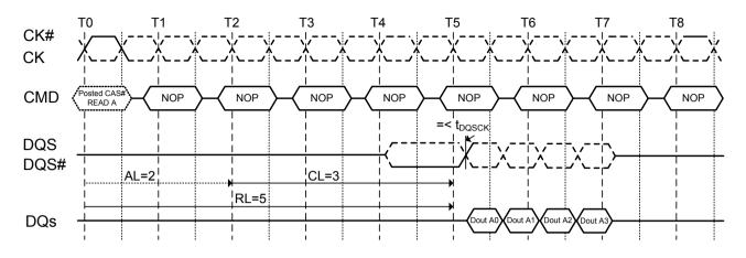
Figure 25. Burst read operation: RL=3 (AL=0, CL=3, BL=8)
