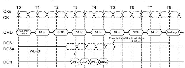
Figure 40. Burst write operation followed by precharge: WL= (RL-1) =3
