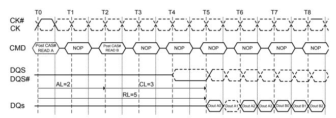
Figure 27. Seamless burst read operation: RL=5, AL=2, CL=3, BL=4
