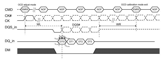
NOTE 1: For proper operation of adjust mode, WL = RL - 1 = AL + CL - 1t<sub>CK</sub> and t<sub>DS</sub>/t<sub>DH</sub> should be met as shown in the figure. NOTE 2: For input data pattern for adjustment, DT0-DT3 is a fixed order and is not affected by burst type (i.e., sequential or interleave)
