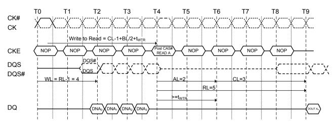
NOTE : The minimum number of clock from the burst write command to the burst read command is [CL-1 + BL/2 +  $t_{WTR}$ ]. This  $t_{WTR}$  is not a write recovery time ( $t_{WR}$ ) but the time required to transfer the 4 bit write data from the input buffer into sense amplifiers in the array.  $t_{WTR}$  is defined in the timing parameter table of this standard.
