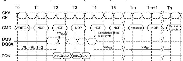
Figure 30. Burst write operation: RL=3 (AL=0, CL=3), WL=2, BL=4
