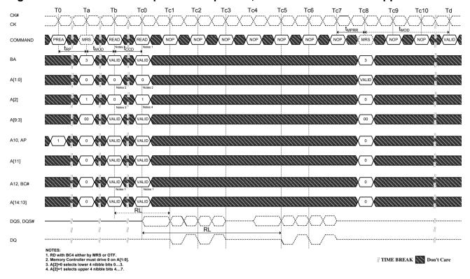
Figure 28. MPR Readout of predefined pattern, BC4 upper nibble then lower nibble
