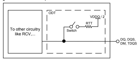
The switch is enabled by the internal ODT control logic, which uses the external ODT pin and other control information. The value of RTT is determined by the settings of Mode Register bits. The ODT pin will be ignored if the Mode Register MR1 and MR2 are programmed to disable ODT and in self-refresh mode.
