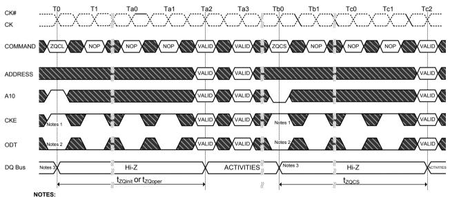
Figure 23. ZQ Calibration Timing
