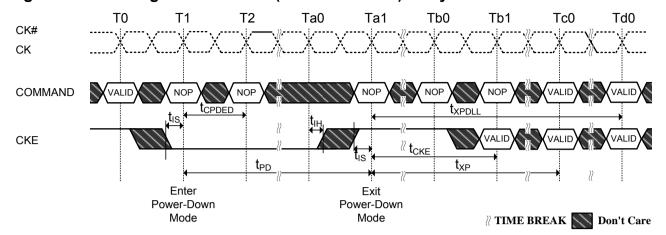
Figure 61. Refresh Command to Power-Down Entry
