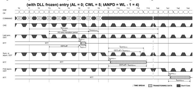
Figure 74. Synchronous to asynchronous transition after Refresh command
