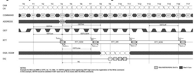
Figure 68. Dynamic ODT: Behavior without write command, AL = 0, CWL = 5
