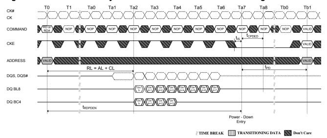
Figure 57. Power-Down Entry after Write with Auto Precharge
