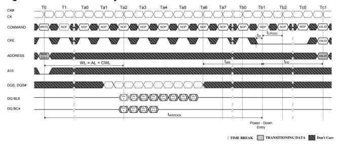
Figure 59. Precharge Power-Down (Fast Exit Mode) Entry and Exit
