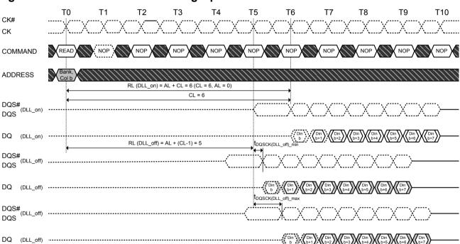
Figure 9. DLL-off mode READ Timing Operation
