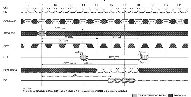
Figure 72. Asynchronous ODT Timings on DDR3 SDRAM with fast ODT transition
