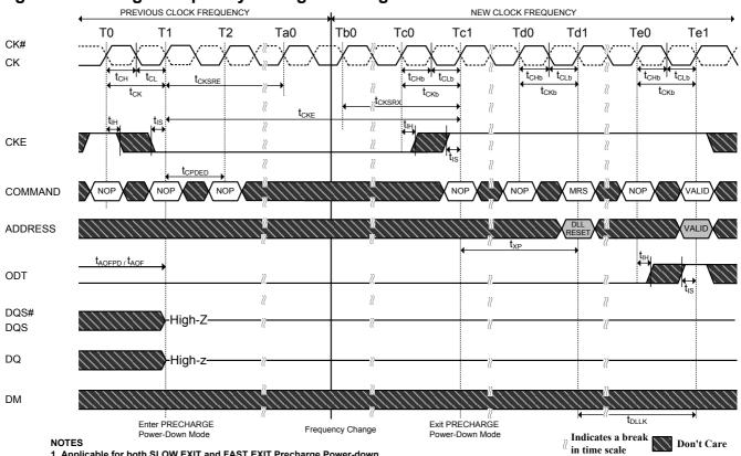
Figure 12. Change Frequency during Precharge Power-down
