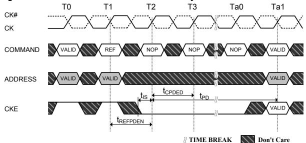
Figure 62. Active Command to Power-Down Entry
