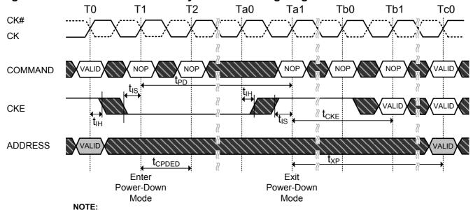
VALID command at T0 is ACT, NOP, DES or PRE with still one bank remaining open after completion of the precharge command.
