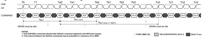
Figure 54. Self-Refresh Entry/Exit Timing
