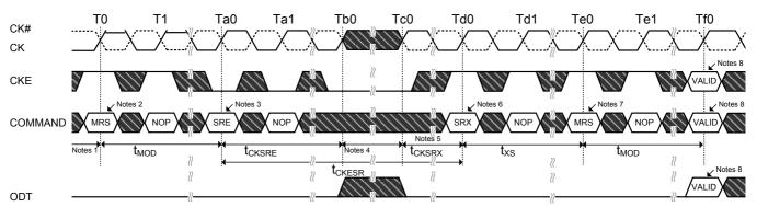
ODT: Static LOW in case RTT\_Nom and RTT\_WR is enabled, otherwise static Low or High
