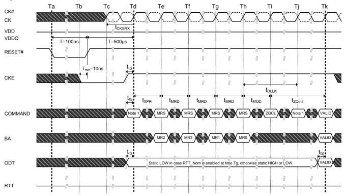
NOTE 1. From time point "Td" until "Tk" NOP or DES commands must be applied between MRS and ZQCL commands.
