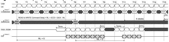
NOTES: 1. RL = 5 (CL = 5, AL = 0), WL = 5 (CWL= 5, AL = 0) 2. DOUT n = data-out from column, DIN b = data-in from column b.
