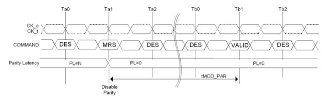
NOTE 1 tMOD\_PAR = tMOD + N; where N is the programmed parity latency.
