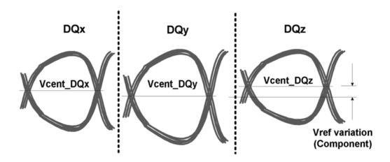
Vcent\_DQ(pin avg) is defined as the midpoint between the largest Vref\_DQ voltage level and the smallest Vref\_DQ voltage level across all DQ pins for a given DRAM component. Each DQ pin Vref level is defined by the center, i.e. widest opening, of the cumulative data input eye as depicted in below. This clarifies that any DRAM component level variation must be accounted for within the DRAM Rx mask. The component level Vref will be set by the system to account for Ron and ODT settings.
