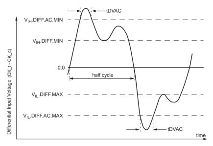
Note 1 Differential signal rising edge from VIL.DIFF.MAX to VIH.DIFF.MIN must be monotonic slope. Note 2 Differential signal falling edge from VIH.DIFF.MIN to VIL.DIFF.MAX must be monotonic slope.
