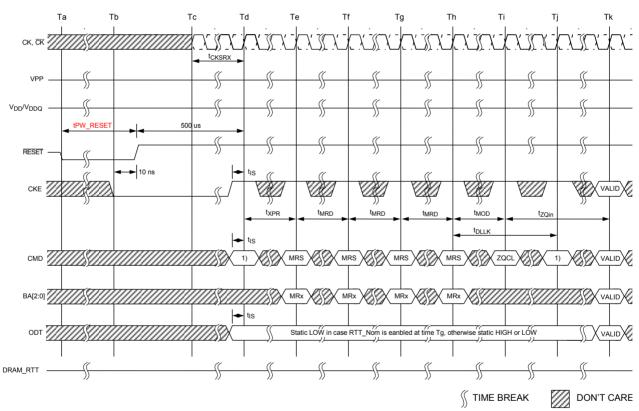
NOTE 1 From the time point Td until Tk, a DES command must be applied between MRS and ZQCL commands.
