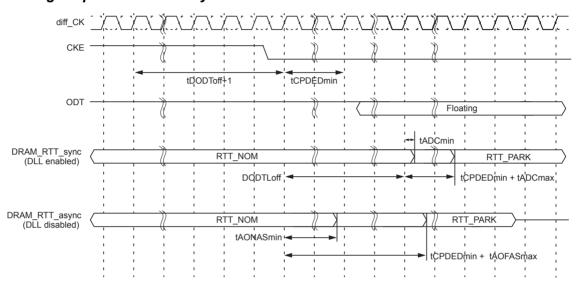
When exit from power down, along with CKE being registered high, ODT input signal must be re-driven and maintained low until tXP is met.
