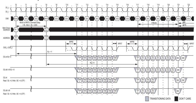
NOTE 1 BL = 8 (or BC = 4 : OTF for Write), RL = 11 (CL = 11, AL = 0), Read Preamble = 1tCK, WL=9 (CWL=9, AL=0), Write Preamble = 1tCK
