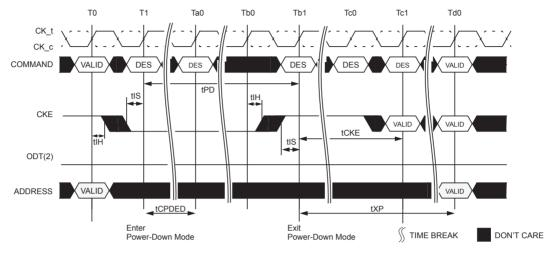
NOTE 1 VALID command at T0 is ACT, DES or Precharge with still one bank remaining open after completion of the precharge command.
