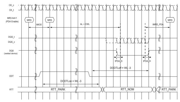
NOTE RTT\_PARK = Enable, RTT\_NOM = Enable, Write Preamble Set = 2tCK and DLL = ON.
