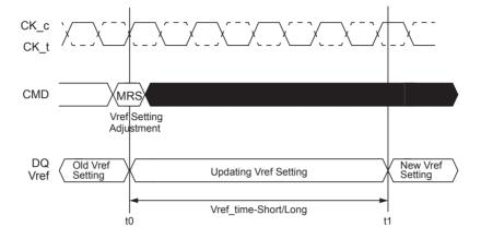
A MRS command to the mode register bits 5:0 of MR6 are used to program the vref value. VrefDQ training mode is enabled/disabledby A7 of MR6 and training range can be selected by A6 of MR6. When VrefDQ training mode is entered/exited, the following parameter needs to be satisfied to prevent current consumption and also stable operation.
