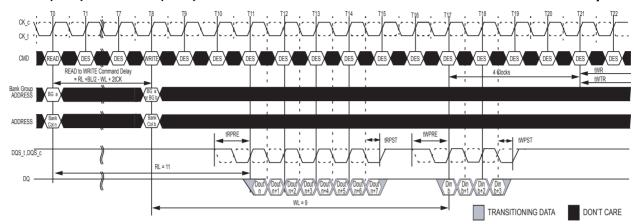
NOTE 1 BL = 8, RL = 11(CL = 11, AL = 0), Read Preamble = 1tCK, WL=9(CWL=9,AL=0), Write Preamble = 1tCK NOTE 2 DOUT n = data-out from column n, DIN b = data-in to column b.
