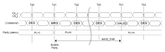
NOTE 1 tMOD PAR = tMOD + N; where N is the programmed parity latency.
