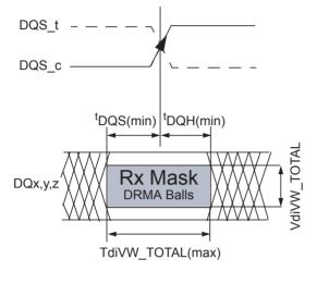
$$\frac{\text{TdiVW\_TOTAL(max)}}{2} = {}^{t}\text{DQS(min)}^{*} = {}^{t}\text{DQH(min)}^{*}$$
