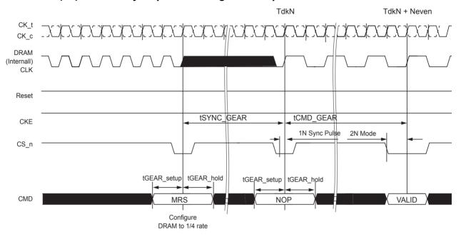
If operation is 1/2 rate(1N) mode before and after self refresh, no MRS command or sync pulse is required during self refresh exit. The min exit delay is tXS, or tXS\_Abort to the first valid command.
