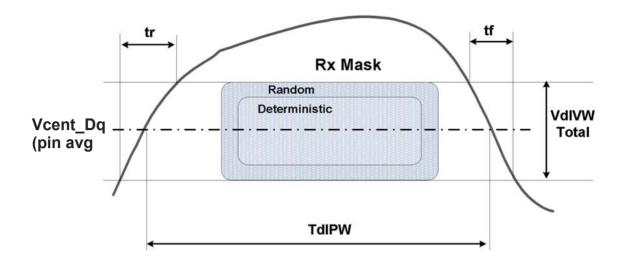
NOTE 1 SRIN\_dIVW=VdIVW\_Total/(tr or tf), signal must be monotonic within tr and tf range.
