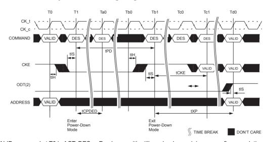
NOTE 1 VALID command at T0 is ACT, DES or Precharge with still one bank remaining open after completion of the precharge command.
