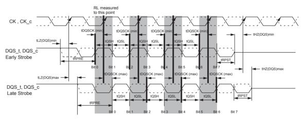
NOTE 1 Within a burst, rising strobe edge will be varied within tDQSCKJ by fixed and constant VDD. However incorporate the device, voltage and temperature variation, rising strobe edge will be varied between tDQSCK(min) and tDQSCK(max).
