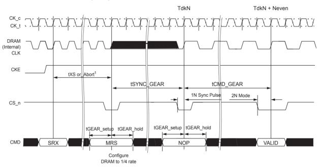
NOTE 1 CKE High Assert to Gear Down Enable Time (tXS, tXS\_Abort) depend on MR setting. A correspondence of tXS/tXS Abort and MR Setting isas follows.
