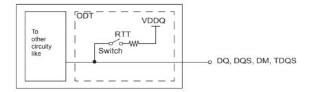
The switch is enabled by the internal ODT control logic, which uses the external ODT pin and Mode Register Setting and other control information, see below. The value of RTT is determined by the settings of Mode Register bits. The ODT pin will be ignored if the Mode Registers MR1 is programmed to disable RTT\_NOM(MR1{A10,A9,A8}={0,0,0}) and in self-refresh mode.
