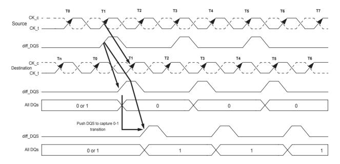
DQS - DQS driven by the controller during leveling mode must be terminated by the DRAM based on ranks populated. Similarly, the DQ bus driven by the DRAM must also be terminated at the controller.
