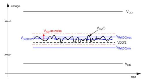
The voltage levels for setup and hold time measurements VIH(AC), VIH(DC), VIL(AC) and VIL(DC) are dependent on VREF. "VREF" shall be understood as VREF(DC), as defined in above figure.
