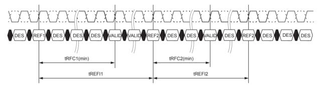
The following conditions must be satisfied before the Refresh rate can be changed. Otherwise, data retention of DDR4 SDRAM cannot be guaranteed.
