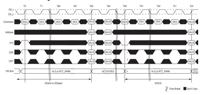
NOTE 1 CKE must be continuously registered high during the calibration procedure.
