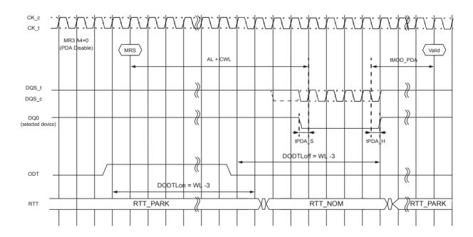
NOTE RTT\_PARK = Enable, RTT\_NOM = Enable, Write Preamble Set = 2tCK and DLL = ON.
