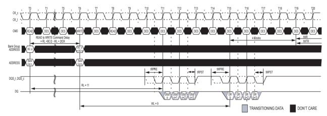
NOTE 1 BC = 4, RL = 11 (CL = 11, AL = 0), Read Preamble = 1tCK, WL = 9 (CWL = 9, AL = 0), Write Preamble = 1tCK NOTE 2 DOUT n = data-out from column n, DIN b = data-in to column b.
