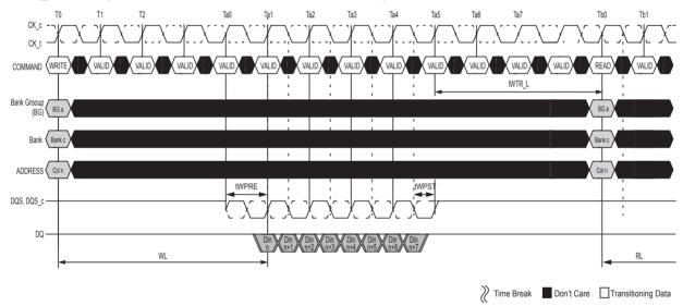
NOTE 1 tWTR\_L: Delay from start of internal write transaction to internal read command to the same Bank Group.
