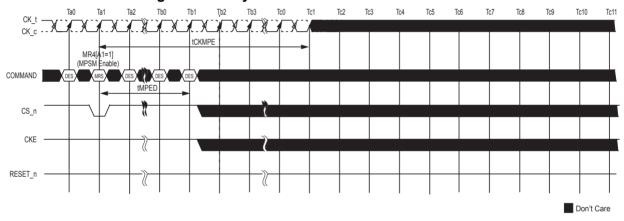
Figure below illustrates the sequence and timing parameters required for the maximum power saving mode with the per DRAM addressability (PDA).
