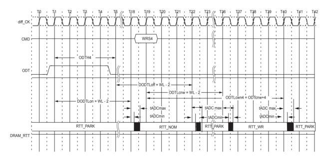
ODT must be held HIGH for at least ODTH4 after assertion (T1). ODTH is measured from ODT first registered HIGH to ODT firstregistered LOW, or from registration of Write command. Note that ODTH4 should be adjusted depending on CRC or 2tCK preamble setting.
