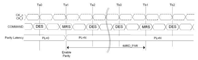
NOTE 1 tMRD\_PAR = tMOD + N; where N is the programmed parity latency.
