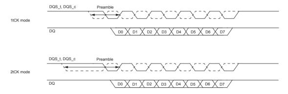
The timing diagrams contained in figure below illustrate 1 and 2 tCK preamble scenarios for consecutive write commands with tCCD timing of 4, 5 and 6 nCK, respectively. Setting tCCD to 5nCK is not allowed in 2 tCK preamble mode.
