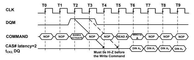
Figure 7. Read to Write Interval (Burst Length ≥ 4, CAS# Latency = 2)
