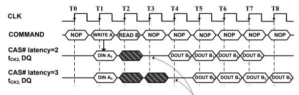
Input data must be removed from the DQ at least one clock cycle before the Read data appears on the outputs to avoid data contention
