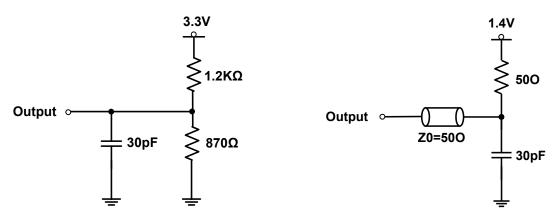
Figure 18.1 LVTTL D.C. Test Load (A)
