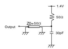
Figure 18.1 LVTTL D.C. Test Load (A)
