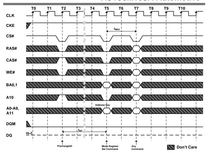
Figure 15. Mode Register Set Cycle
