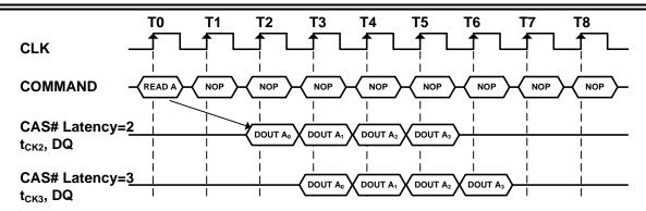
Figure 4. Burst Read Operation (Burst Length = 4, CAS# Latency = 2, 3)
