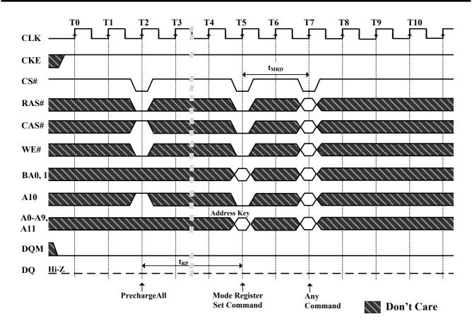
Figure 15. Mode Register Set Cycle
