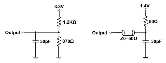
Figure 18.1 LVTTL D.C. Test Load (A)
