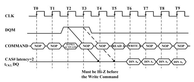
Figure 6. Read to Write Interval (Burst Length ≥ 4, CAS# Latency = 2)
