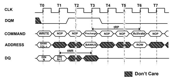
**Note:** The DQMs can remain low in this example if the length of the write burst is 1 or 2.
