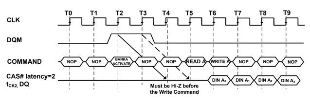
Figure 6. Read to Write Interval (Burst Length  $\geq$  4, CAS# Latency = 2)
