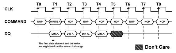
A write burst without the auto precharge function may be interrupted by a subsequent Write, BankPrecharge/PrechargeAll, or Read command before the end of the burst length. An interrupt coming from Write command can occur on any clock cycle following the previous Write command (refer to the following figure).
