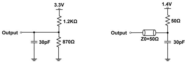
Figure 18.1 LVTTL D.C. Test Load (A)
