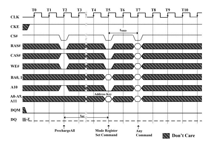
Figure 15. Mode Register Set Cycle
