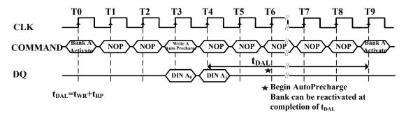
Figure 14. Burst Write with Auto-Precharge (Burst Length = 2)
