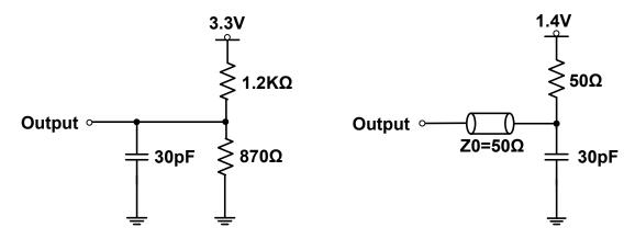
Figure 18.1 LVTTL D.C. Test Load (A)
