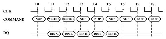
Figure 11. Write Interrupted by a Write (Burst Length = 4)
