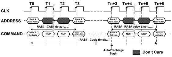
Figure 3. BankActivate Command Cycle (Burst Length = n)
