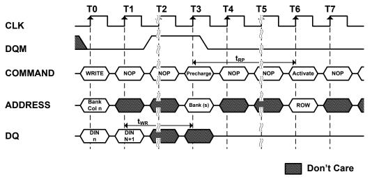
Note: The DQM can remain low in this example if the length of the write burst is 1 or 2.
