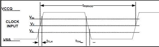
Note 1:  $V_{IH}$  denote  $V_{IH}$ (min.) and  $V_{IL}$  denotes  $V_{IL}$ (max.). Note 2:  $V_T$ =0.975V – Clock Threshold, indicates clock reference point for timing measurements.
