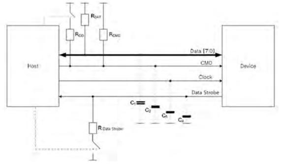
The  $R_{0D}$  is switched on and off by the host synchronously to the open-drain and push-pull mode transitions. The host does not have to have open drain drivers, but must recognize this mode to switch on the  $R_{0D}$ .  $R_{DAT}$  and  $R_{CMD}$  are pull-up resistors protecting the CMD and the DAT lines against bus floating device when all device drivers are in a high-impedance mode.
