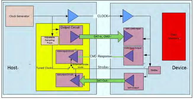
Figure 7: HS400 Host and Device block diagram
