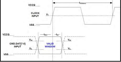
Note 1:  $t_{ISU}$  and  $t_{IH}$  are measured at  $V_{IL}$ (max.) and  $V_{IH}$ (min.). Note 2:  $V_{IH}$  denote  $V_{IH}$ (min.) and  $V_{IL}$  denotes  $V_{IL}$ (max.).
