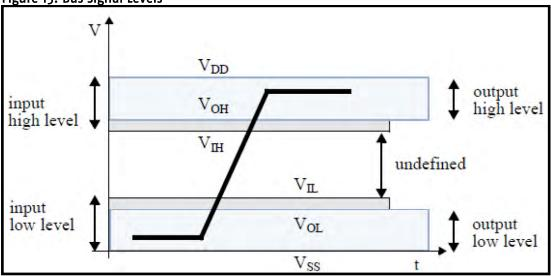
Figure 15: Bus Signal Levels
