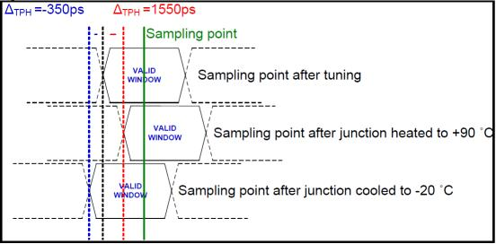
Implementation Guide: Host should design to avoid sampling errors that may be caused by the  $\Delta_{TPH}$  drift. It is recommended to perform tuning procedure while Device wakes up, after sleep. One simple way to overcome the  $\Delta_{TPH}$  drift is by reduction of operating frequency.
