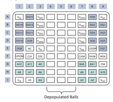
Note: 1. The balls at A4, A5, and A6 are absent from the physical package. They are included to illustrate that rows 4, 5, and 6 exist, but contain no solder balls.
