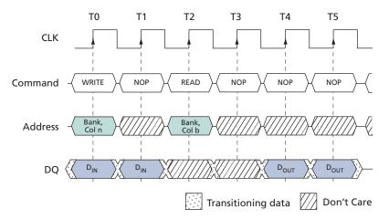
Note: 1. The WRITE command can be issued to any bank, and the READ command can be to any bank. DQM is LOW. CL = 2 for illustration.
