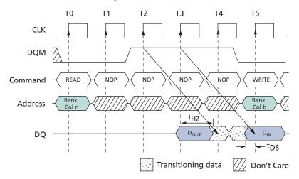
Note: 1. CL = 3. The READ command can be issued to any bank, and the WRITE command can be to any bank.
