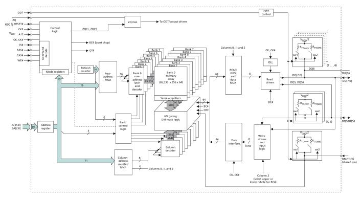
Figure 4: 1 Gig x 8 Functional Block Diagram
