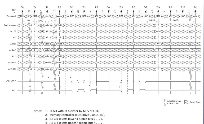
Figure 60: MPR System Read Calibration with BC4: Lower Nibble, Then Upper Nibble
