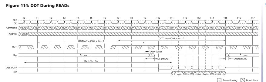
Note: 1. ODT must be disabled externally during READs by driving ODT LOW. For example, CL = 6; AL = CL - 1 = 5; RL = AL + CL = 11; CWL = 5; ODTLon = CWL + AL - 2 = 8; ODTLoff = CWL + AL - 2 = 8. R<sub>TT,nom</sub> is enabled. R<sub>TT(WR)</sub> is a "Don't Care."
