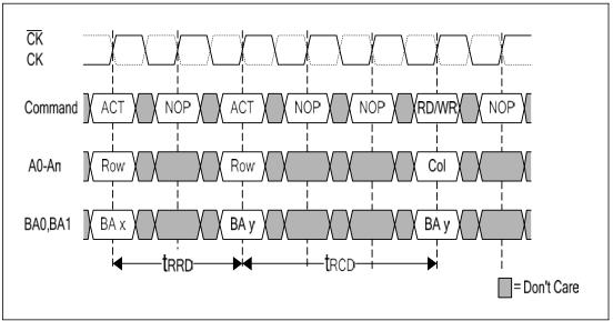
Figure 11 — Bank Activation Command Cycle
