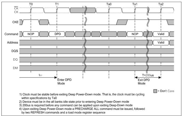
Figure 38 — Deep Power-Down Entry and Exit
