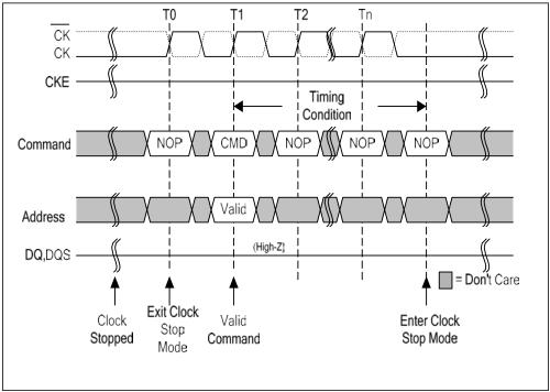
Figure 39 — Clock Stop Mode Entry and Exit
