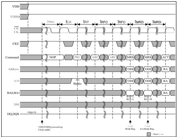
Figure 5 — Initialization Waveform Sequence
