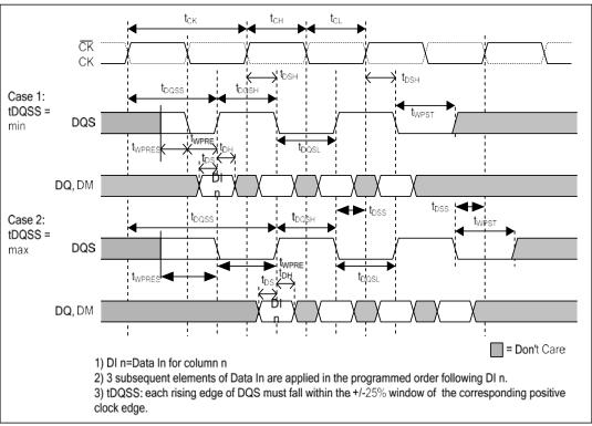
Figure 23 — Basic Write Timing Parameters
