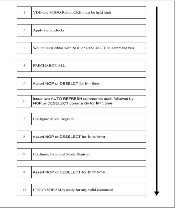
Figure.4 — Flow Diagram
