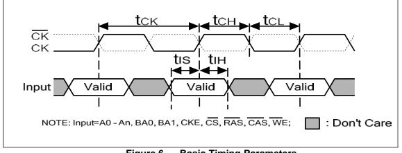
Figure.6 — Basic Timing Parameters
