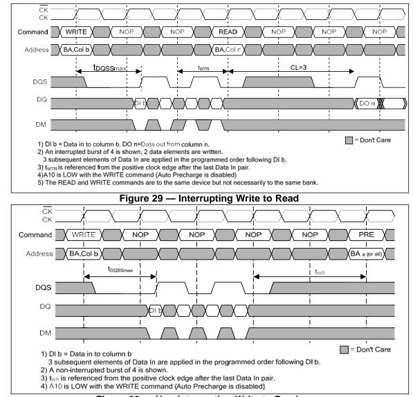
Figure 30 — Non-Interrupting Write to Precharge
