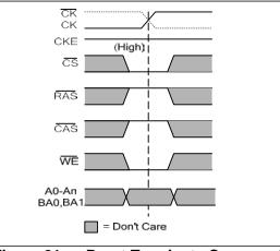
Figure 21 — Burst Terminate Command
