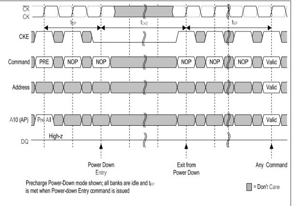
Figure 37 — Power-Down Entry and Exit
