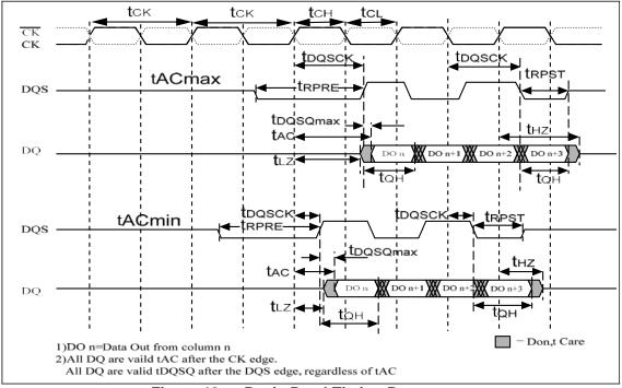
Figure 13 — Basic Read Timing Parameters
