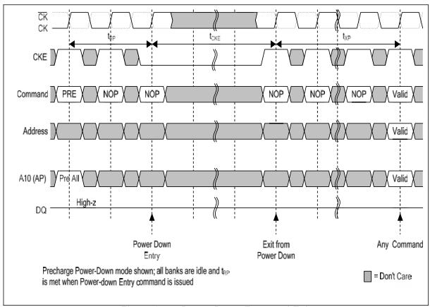
Figure 37 — Power-Down Entry and Exit
