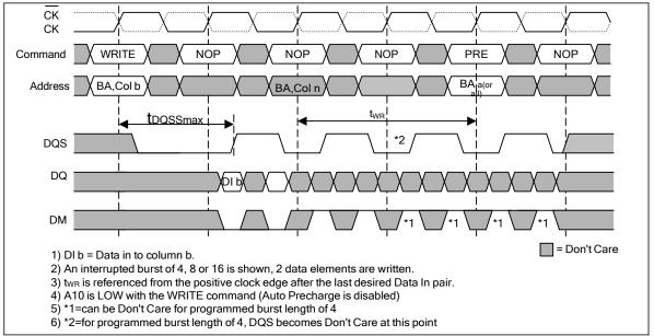
Figure 31 — Interrupting Write to Precharge
