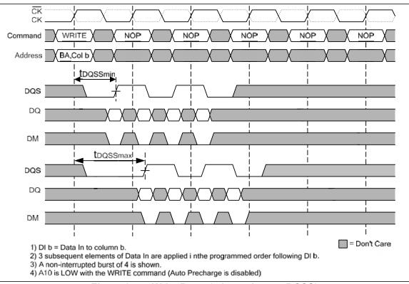
Figure 24 — Write Burst (min. and max. tDQSS)
