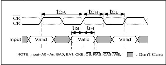
Figure.6 — Basic Timing Parameters
