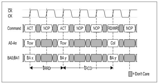
Figure 11 — Bank Activation Command Cycle
