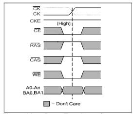
Figure 21 — Burst Terminate Command
