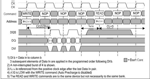
Figure 28 — Non-Interrupting Write to Read
