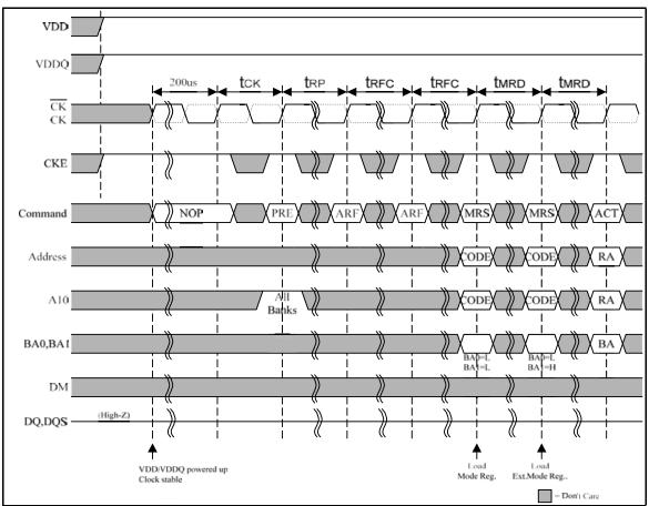
Figure 5 — Initialization Waveform Sequence
