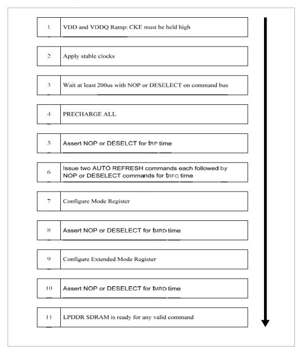
Figure.4 — Flow Diagram
