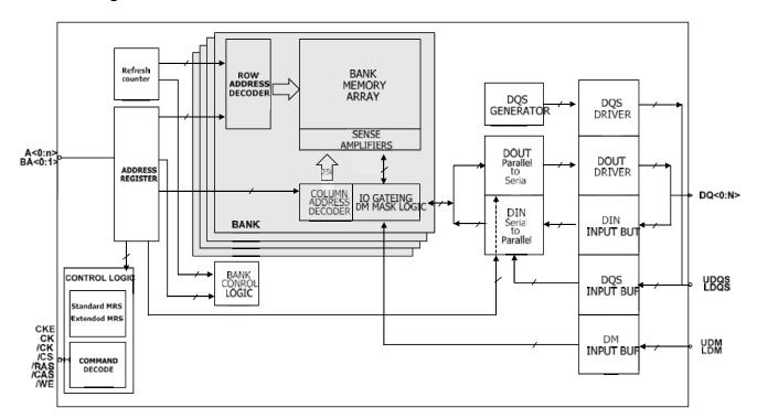
Figure.2 — Block Diagram
