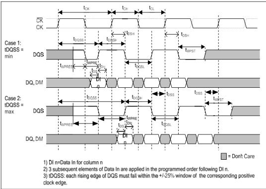
Figure 23 — Basic Write Timing Parameters
