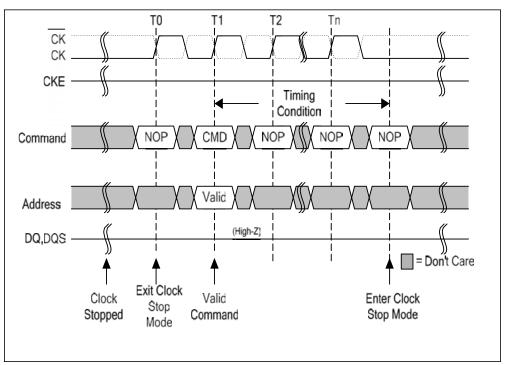
Figure 39 — Clock Stop Mode Entry and Exit
