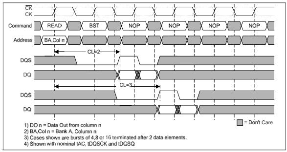
Figure 18 — Terminating a Read Burst
