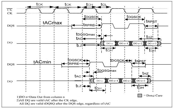
Figure 13 — Basic Read Timing Parameters
