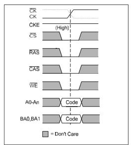
Figure 8 — Mode Register Set Command
