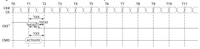
Note: 1. CKE can go LOW at tHCKE after the clock on which the ACTIVATE command is registered.
