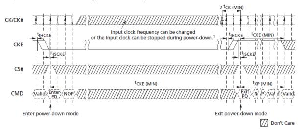
Note: 1. Input clock frequency can be changed or the input clock stopped during power-down, provided that the clock frequency is between the minimum and maximum specified frequencies for the speed grade in use, and that prior to power-down exit, a minimum of two stable clocks complete.
