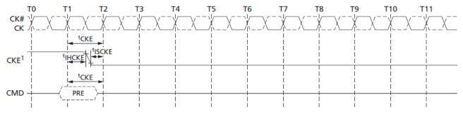
Note: 1. CKE can go LOW tHCKE after the clock on which the PRECHARGE command is registered.
