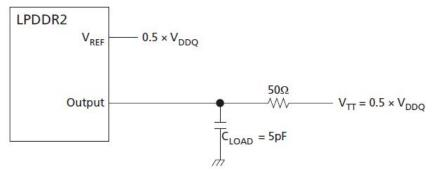
Note: 1. All output timing parameter values (tDQSCK, tDQSQ, tQHS, tHZ, tRPRE etc.) are reported with respect to this reference load. This reference load is also used to report slew rate.
