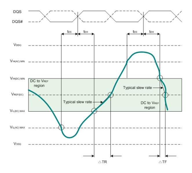
Hold slew rate falling signal =
