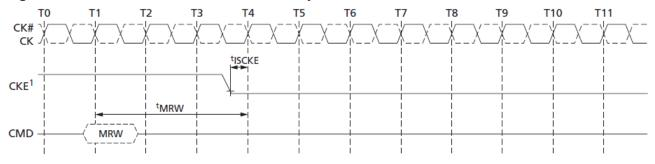
Note: 1. CKE can be registered LOW tMRW after the clock on which the MRW command is registered.
