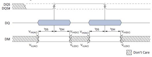
Figure 22: Write Data Mask - Second Data Bit Masked
