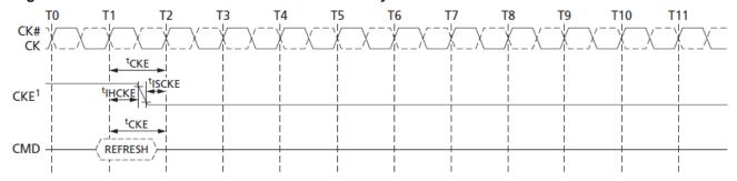
Note: 1. CKE can go LOW tIHCKE after the clock on which the REFRESH command is registered.
