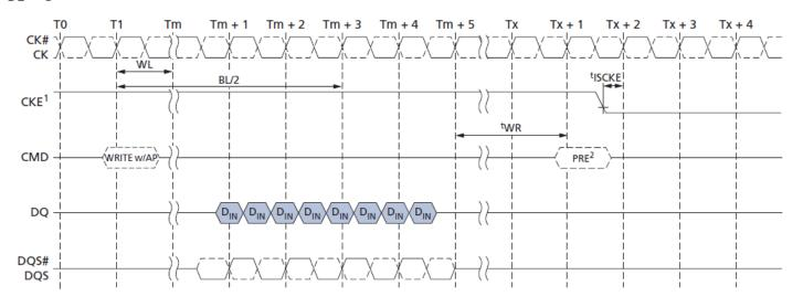
Notes: 1. CKE can be registered LOW at (WL + 1 + BL/2 + RU(tWR/tCK + 1) clock cycles after the WRITE command is registered.
