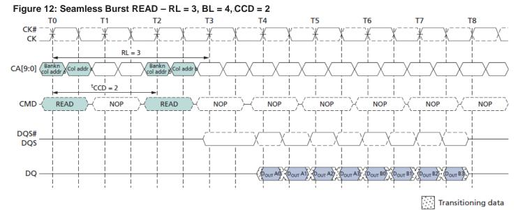
A seamless burst READ operation is supported by enabling a READ command at every other clock cycle for BL = 4 operation, every fourth clock cycle for BL = 8 operation, and every eighth clock cycle for BL = 16 operation. This operation is supported as long as the banks are activated, whether the accesses read the same or different banks.
