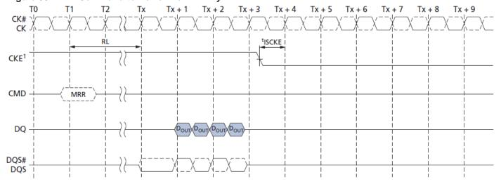
Note: 1. CKE can be registered LOW at (RL + RU(tDQSCK/tCK)+ BL/2 + 1) clock cycles after the clock on which the MRR command is registered.
