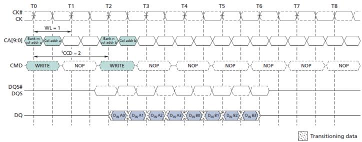
Note: 1. The seamless burst WRITE operation is supported by enabling a WRITE command every other clock for BL = 4 operation, every four clocks for BL = 8 operation, or every eight clocks for BL = 16 operation.
