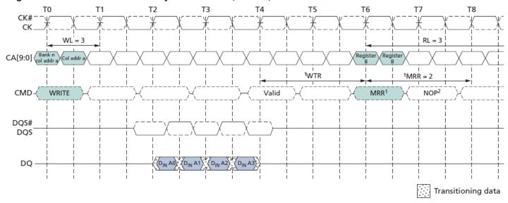
$Notes: 1. \ The \ minimum \ number \ of \ clock \ cycles \ from \ the \ burst \ WRITE \ command \ to \ the \ MRR \ command \ is \ [WL+1+BL/2+RU(tWTR/tCK)].$
