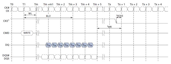
Note: 1. CKE can be registered LOW at (WL + 1 + BL/2 + RU(tWR/tCK)) clock cycles after the clock on which the WRITE command is registered.
