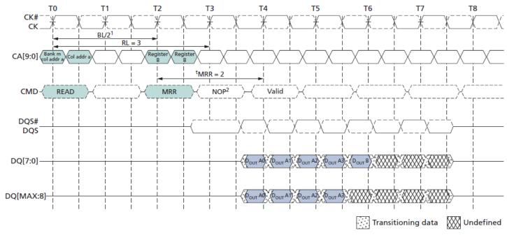
Notes: 1. The minimum number of clock cycles from the burst READ command to the MRR command is BL/2.
