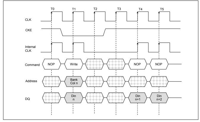
Figure 23. Clock Suspend During Write Burst
