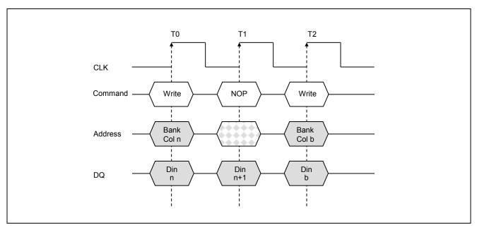
Figure 16. Write to Write - Transition from a burst of 2 to a single write
