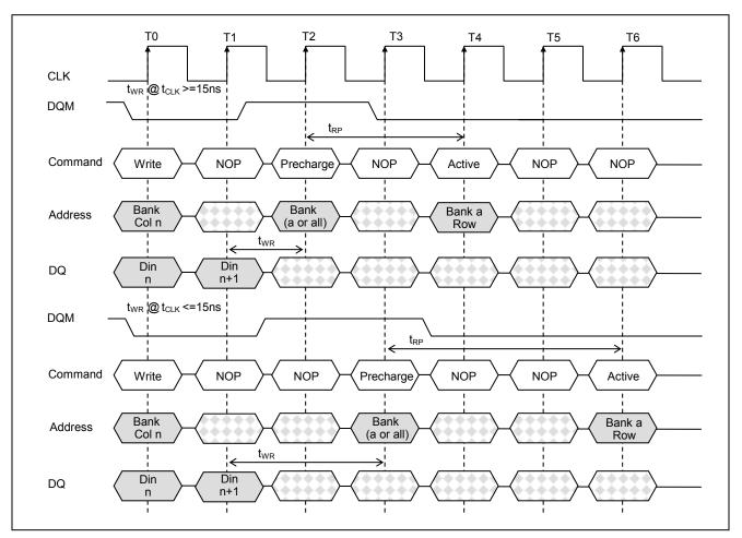
Figure 19. Write to Precharge
