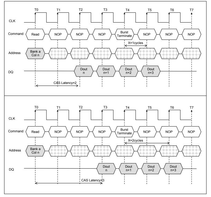
Figure 10. Terminating a Read Burst
