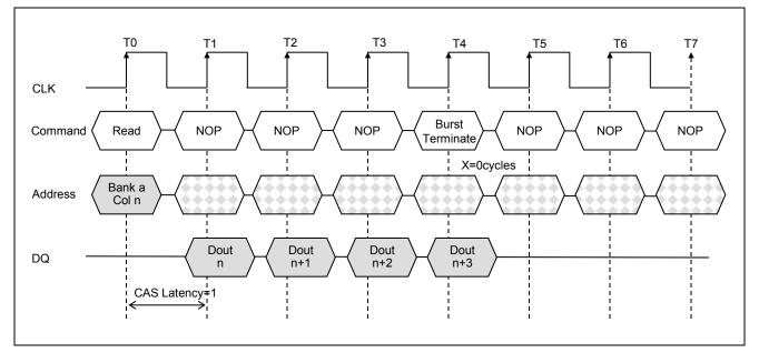
Figure 10. Terminating a Read Burst
