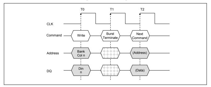
Figure 20. Terminating a Write Burst
